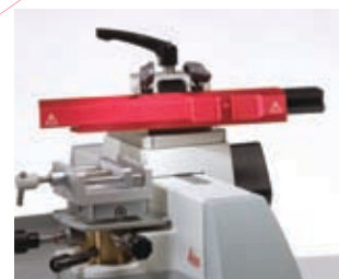
Knife holder SN for standard knives or disposable blade rails
