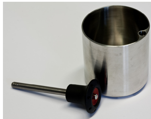
Sample Container with quick release pin
