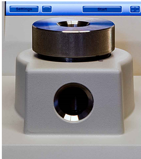
Sample Container with quick release pin
