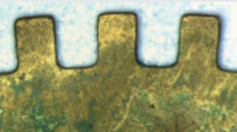
Oxidation on gear wheel
