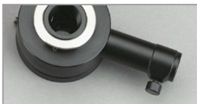
Coaxial incident light housing for fiber-optic light
